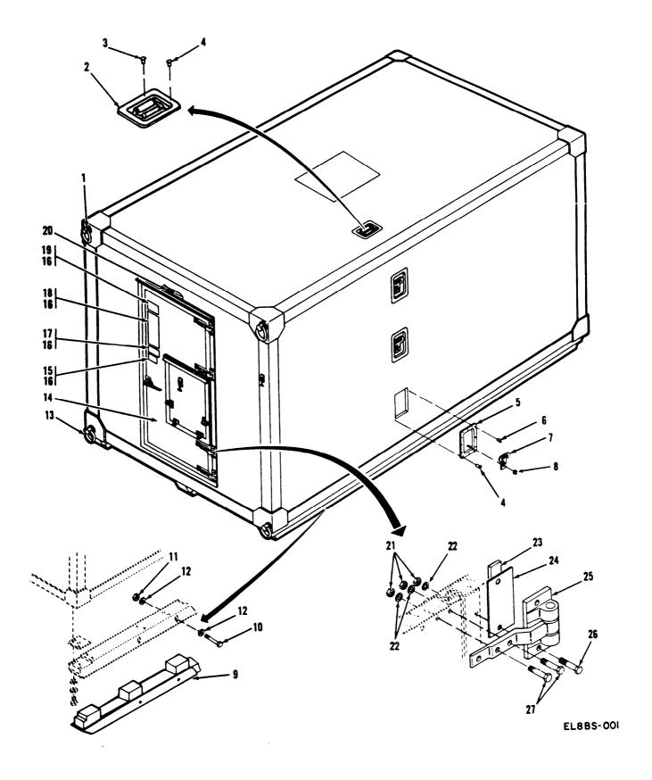
Figure 1. Shelter, Electrical Equipment S-280C/G (Sheet 1 of 2) 4.1
