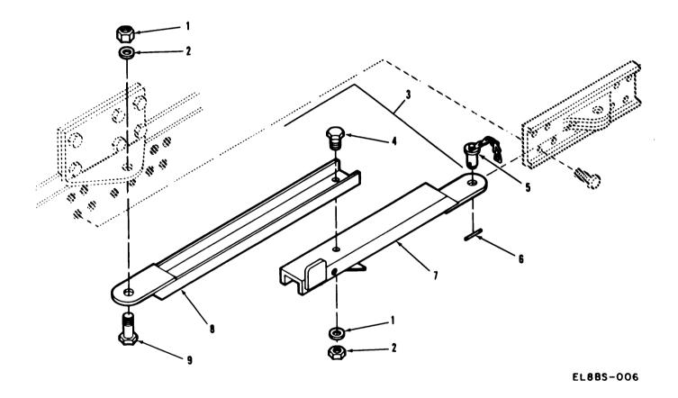
Figure 4. Door Brace Assembly.
